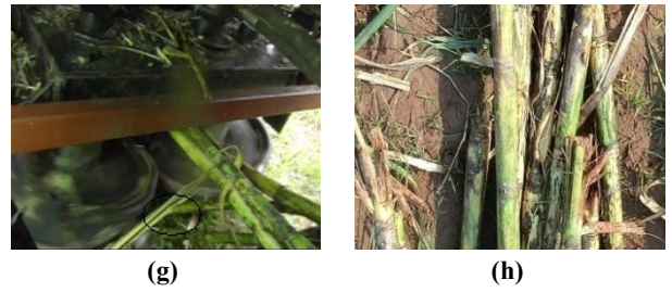
Figure 10(a)-(h). Part of video screenshots about lifter spiral coated with smooth-surfaced rubber and the drum without rubber t_a=44\text{s} t_b=50\text{s} t_c=54\text{s} t_d=78\text{s} t_e=119\text{s} t_f=131\text{s} t_g=148\text{s}
