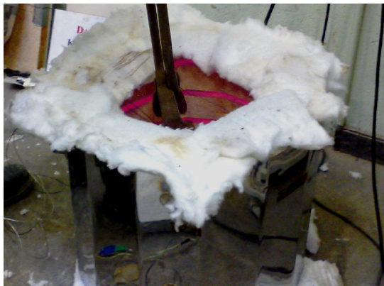
Figure 2. Heating of LFC specimens in an electric furnace to predetermined temperatures
