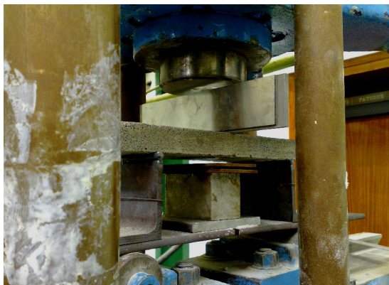
Figure 3. Set up for three point bending test
