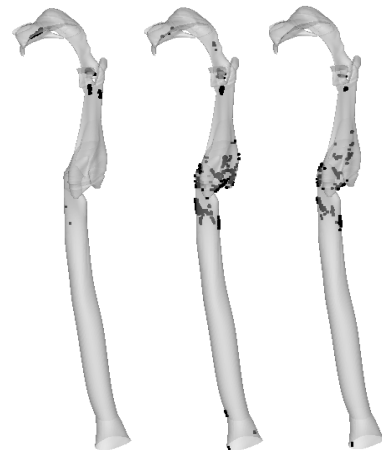
Figure 9. Depositions pattern of 3, 7 and 16 \mu m particles on the walls of the upper airways in the breathing rate of 15 l/min
