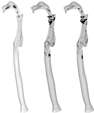
Figure 10. Depositions pattern of 3, 7 and 16\mu\text{m} particles on the walls of the upper airways in the breathing rate of 30 l/min.
