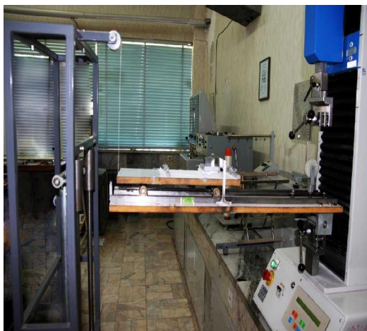
Figure 3. Diagram of the new device for measuring the frictional force with designed escalator
