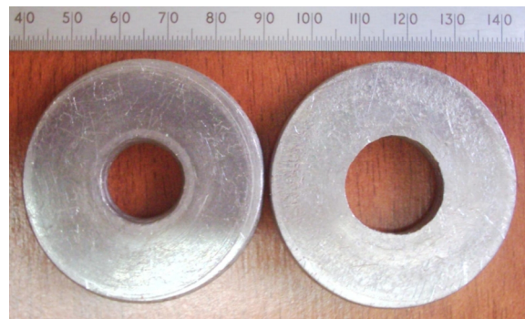
Figure 4. The specimens after ring tests using different lubricants. (Left): Emery powder. (Right): Grease
