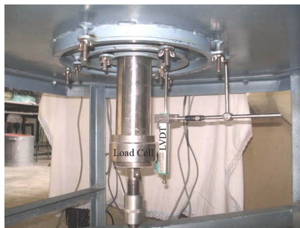
Figure 6. Detail of the trapdoors, load cell and displacement gauge.
