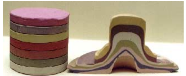
Figure 4. The billet and deformed plasticine specimen.
