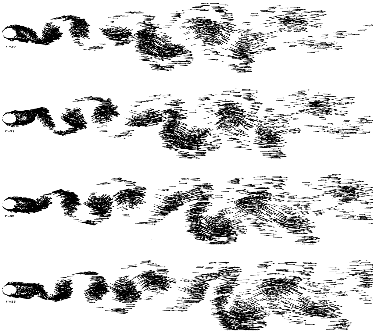
Figure 11. Positions and velocities of vortex elements downstream versus time at Re=3000 .
