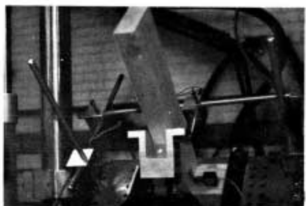
Figure 7. The Set Up of the Clip-on-Gage Mounting.
