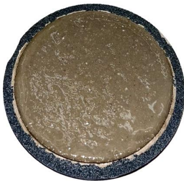
Figure 1. Formed filter cake after high-pressure and high-temperature filter press
