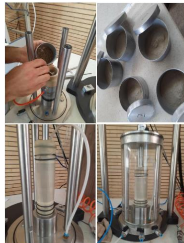
Figure 6. Sample preparation in Triaxial device
