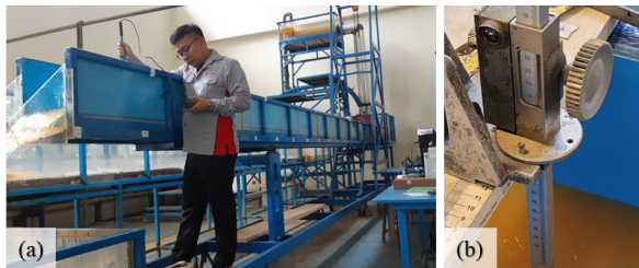
Figure 7. (a) Flow velocity measurement using a flow meter (left) and (b) flow depth measurement using a point gauge (right)
