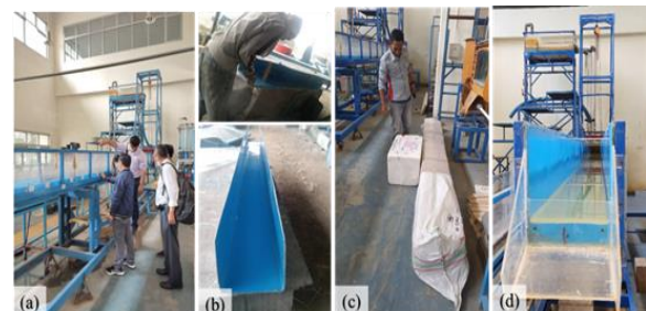
Figure 5. (a) Measurements, (b) manufacturing, (c) packaging, and (d) installation of the GFRP material into the flume
