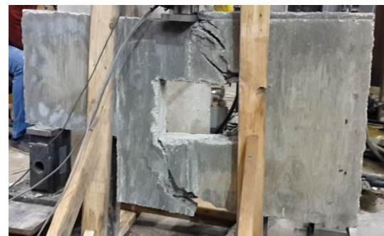
Figure 11. The failure mode in Specimen 2
