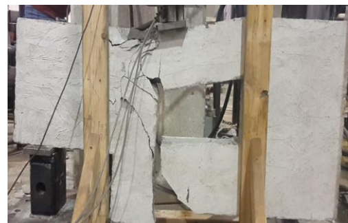
Figure 12. The failure mode in Specimen 3
