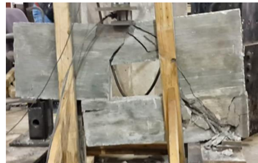
Figure 10. The failure mode in Specimen 1
