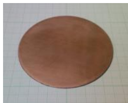
Figure 5. Disc sample with a diameter of 58 mm
