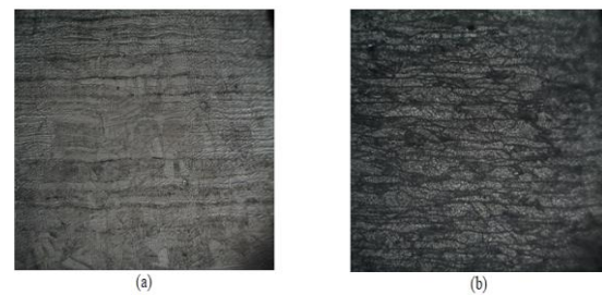
Figure 1. Microstructure of (a) steel 304 (b) aluminum 5052 at scale 40x
