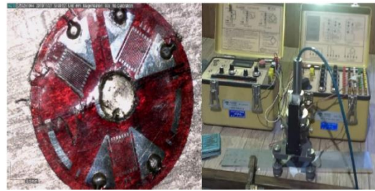
Figure 24. Central drilling test with strain gauge installation
