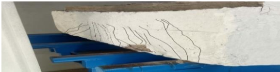
Figure 13. Beam failure and crack distribution of RCJ2 beam
