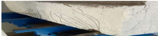
Figure 11. Beam failure and crack distribution of RCJ0 beam
