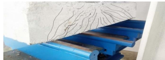
Figure 9. The failure mode of control beam
