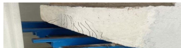
Figure 15. Beam failure and crack distribution of RCJ4 beam
