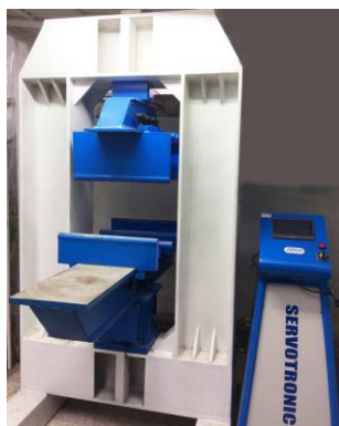
Figure 7. Bending jack used in the beams flexural load test
