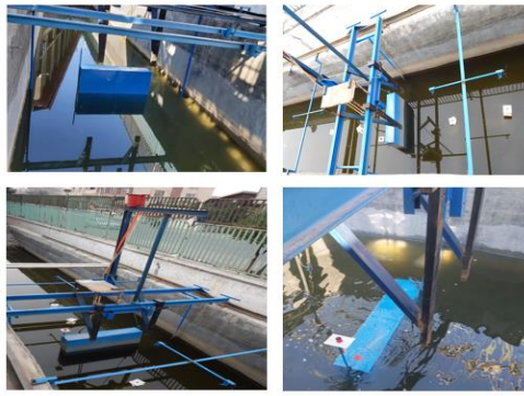
Figure 2. Views of a 1: 8 scale OWSC wave energy converter made in a laboratory
