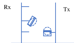
Figure 12. The Position of Receiver Antenna with 70° inclination
