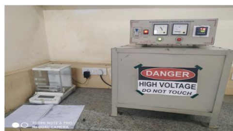
Figure 2. The silicon carbide tube furnace used for high temperature corrosion studies
