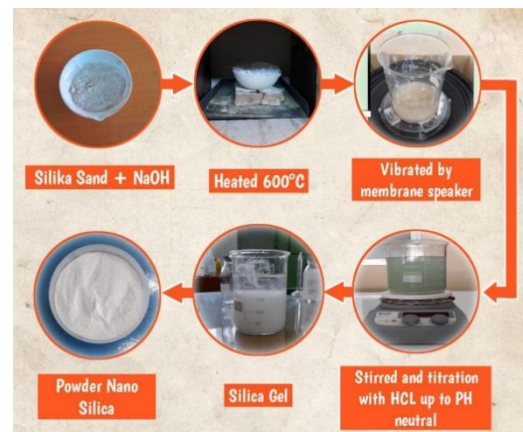
Figure 1. Schematic illustration of the synthesis method of SNP
