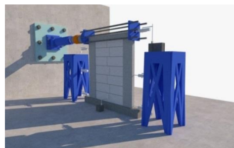
Figure 3. Setting up of RC frame infilled with prefabricated plain foamed concrete blocks specimen
