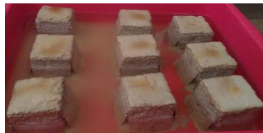
Figure 8. Spalling of RPC Samples with 60 days exposure
