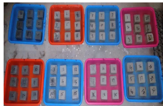
Figure 1. Specimens immersed in H 2 SO 4 solution
