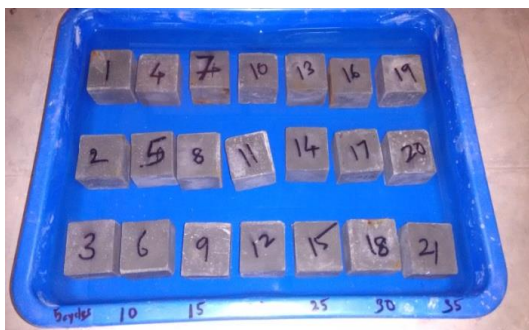
Figure 2. Specimens immersed in \text{Na}_2\text{SO}_4 solution
