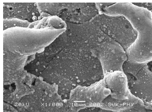
Figure 7. Micro- craks of machined surface
