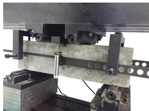
Figure 4. Fibrous concrete prism under flexural testing
