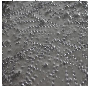
(b) Uniform distribution fibres after mixing procedure Figure 2. Mixer and a sample of a mixed matrix
