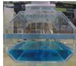
Figure 1. Prismatic tank with 25% filling ratio [11]
