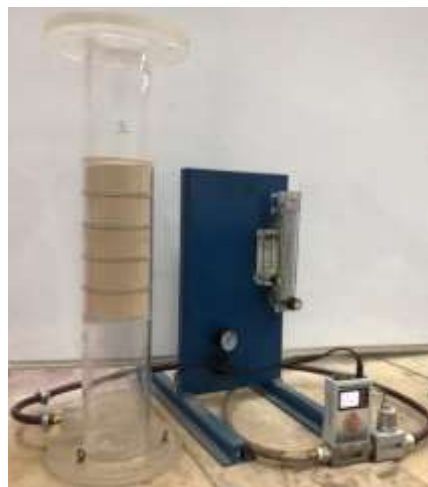
Figure 1. ADMFB filled with silica sand and connected to the mass flow controller (not covered in the wool glass yet)
