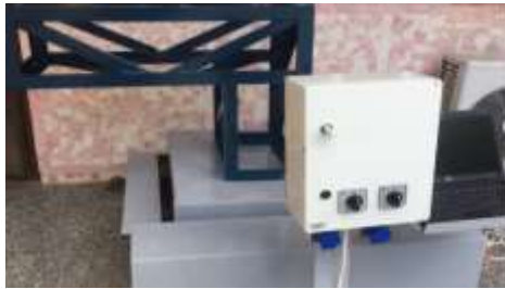
Figure 3. Shaking table developed as experimental rig
