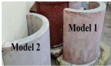
Figure 5. Concrete arch dam models
