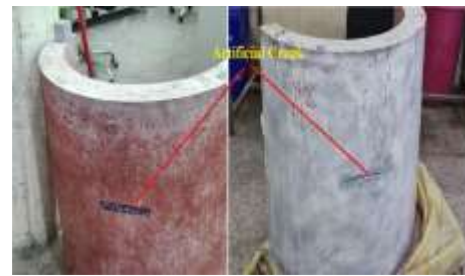
Figure 7. Concrete arch dam with artificial crack
