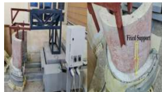
Figure 8. Concrete arch dam model with fixed support
