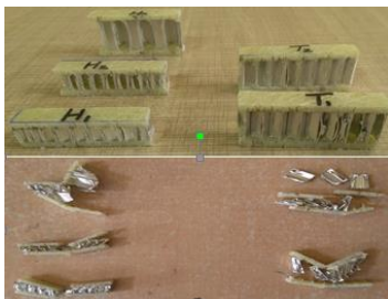
Figure 3. Sandwich structure before and after Charpy impact
