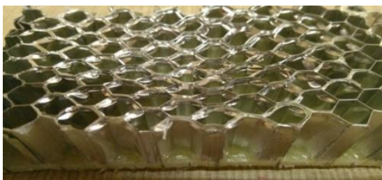
Figure 9. Plastic deformation of honeycomb
