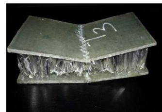
Figure 6. Damaged honeycomb sandwich after CAI
