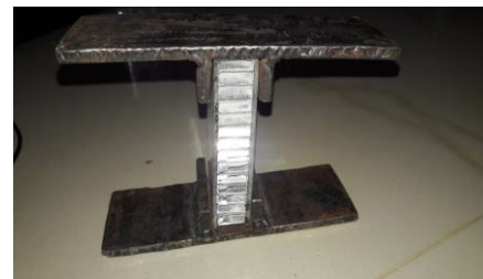
Figure 4. Test fixture for CAI
