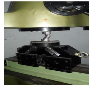
Figure 5. Specimen under compression in UTM with the test fixture
