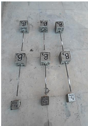
Figure 4. Casted BIS pull-out specimens
