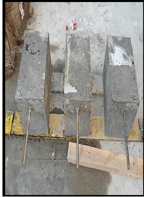
Figure 8. Casted beam-end specimens
