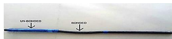
Figure 7. PSWC rebar with bonded and un-bonded regions
