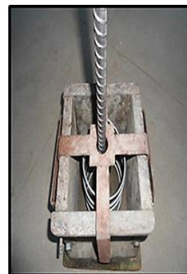
Figure 3. Arrangement of mould for casting pull-out specimen
