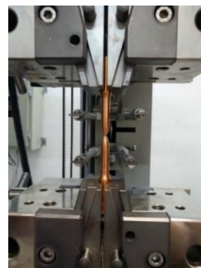
Figure 2. Setup of tensile test equipment
