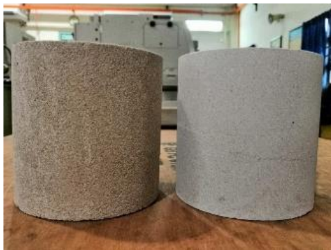
Figure 2. One of the rock samples for Indiana limestone (left) and Carthage marble (right) used in rock cutting experiment
