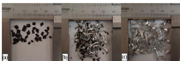
Figure 13. Cast iron chips (a), Bimetallic parts chips (b) and Aluminum chips (c)
