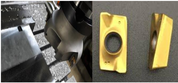
Figure 3. Tool inserts (right) and tool holder (left) for face milling
