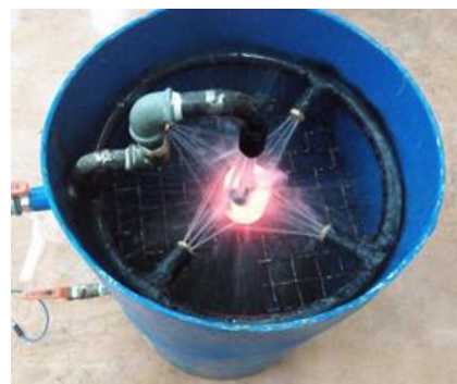
Figure 1. Illustrating the water spray cooling rig
