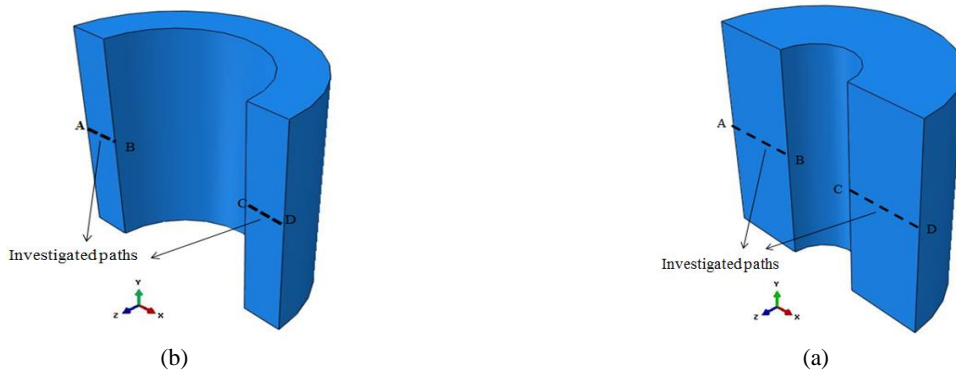
Figure 8. Comparing paths on samples with, (a) 20mm inner diameter, (b) 40mm inner diameter
