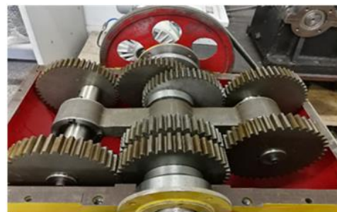
Figure 1. Reversing device of planetary gear train with elliptic cylinder gears
