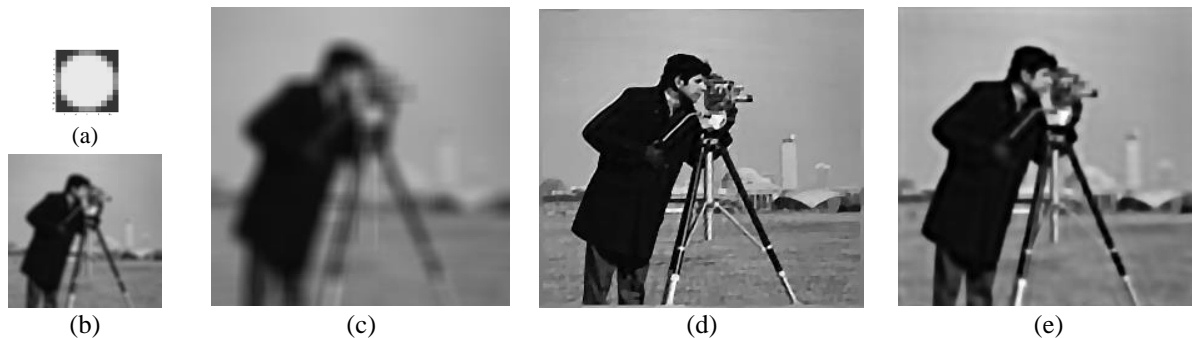
Figure 2. (a) Applied blur kernel ( 11 \times 11 ), (b) One of LR image, (c) Blur HR image, (d) Reconstructed HR image (SSIM: 0.8381), (e) Result of [16] (SSIM: 0.7630)
