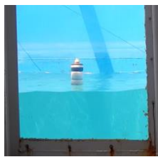
Figure 6. Buoy in the wave tank to measure the wave characteristics.
