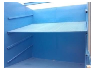
Figure 3. The damper system of the wave tank
